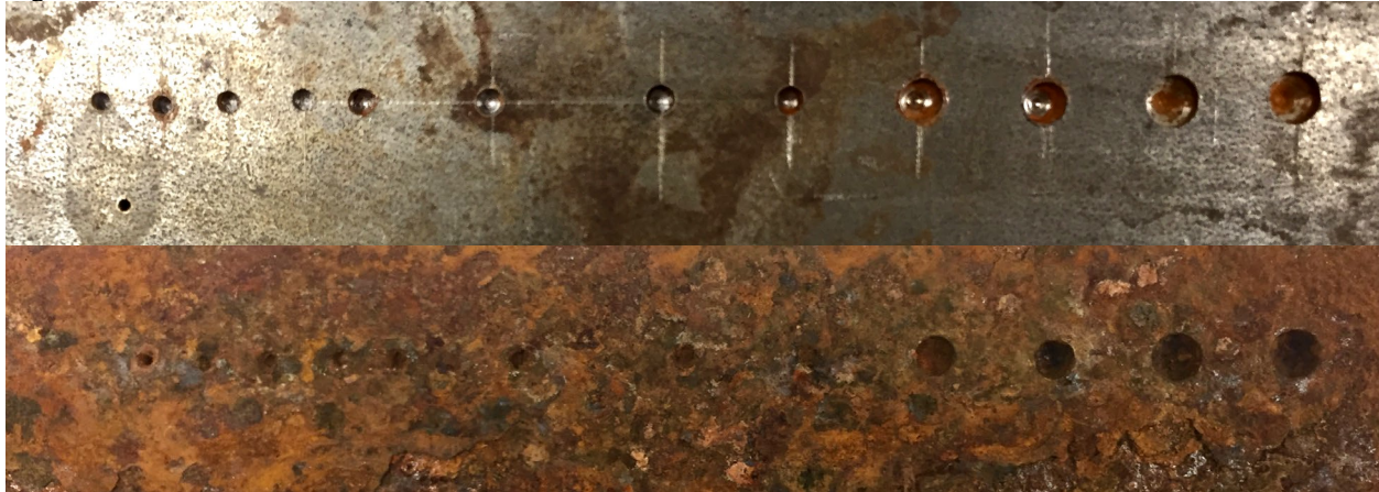
Figure 1: The top picture is the initial carbon steel plate and the one below is the same part at the end of the galvanic corrosion test.
