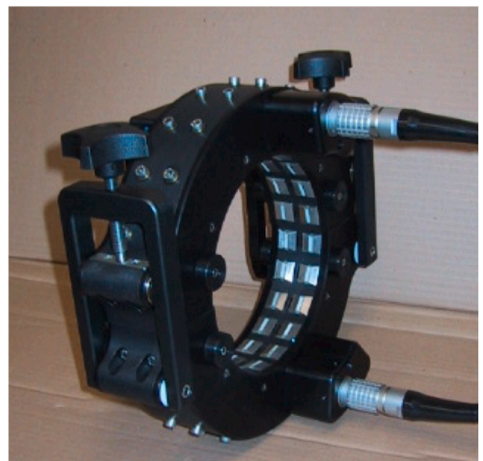
Fig. 13. Solid transducer assembly for 8-inch pipe showing array of dry-coupled piezoelectric transducers (Guided Ultrasonics Ltd [136]).
