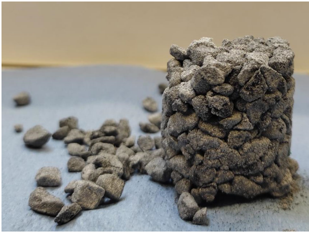
Fig. 5 Agglomerated grains after 10 cycles (Video 1 presented as supplementary material is a good visualization for the swelling and shrinkage phenomena in bed as it is cycled.)
