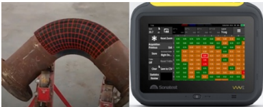
0° Manual UT Spot Reading Grid
