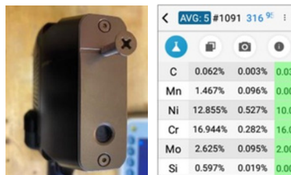
Figure 4 SciAps Z-902 Carbon analysis of 1/8" wire, 316
