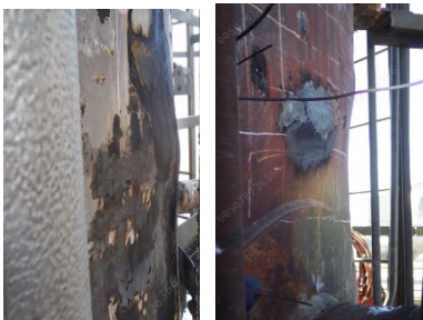
Figure-2 Distortion in a vertical vessel resulted from improper application of local PWHT [2]
